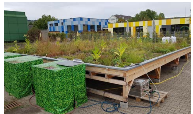
Fig. 27: The "EffIN-Green Project" covers various aspects, including the evaporation performance of extensive greening. Source: BuGG
