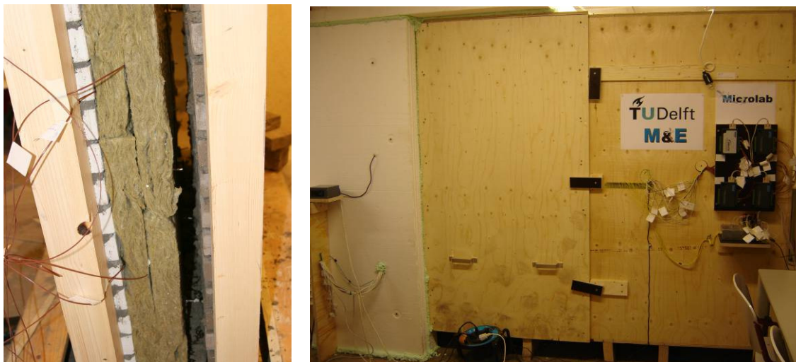
Figures 5 and 6: left photo; the constructed wall element with thermocouples. Right photo; experimental set up called “Hotbox” to simulated environmental conditions.
